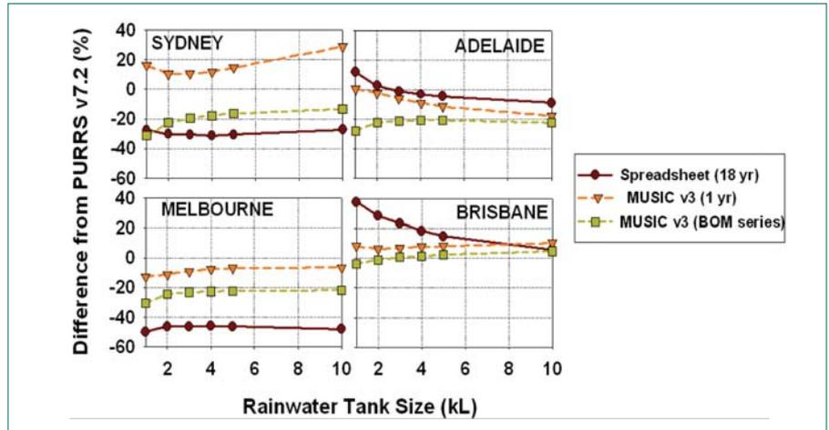
**Figure 6.** Difference in results from the common use of Spreadsheet and MUSIC in comparison to PURRS results.
