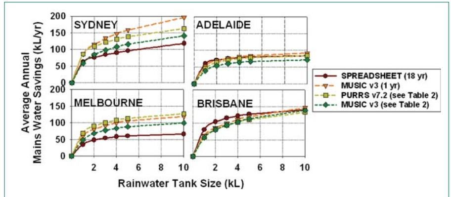
**Figure 4.** Comparisons of mains water savings derived from common uses of the selected models.
