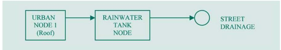
**Figure 3.** Generic structure of MUSIC models used to simulate rainwater harvesting from roofs.
