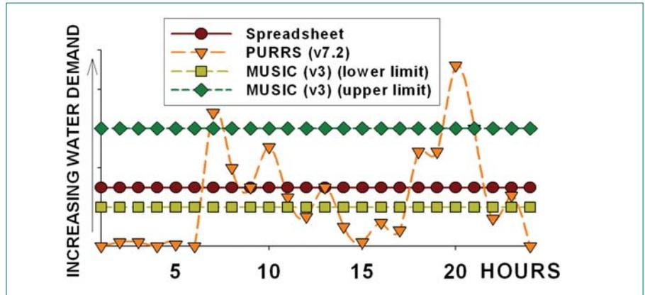
Figure 8: Water use patterns used in the selected models.
