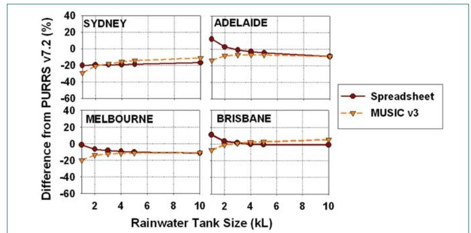
**Figure 7.** Difference in results from the use of equal rainfall durations in Spreadsheet and MUSIC when compared to PURRS.
