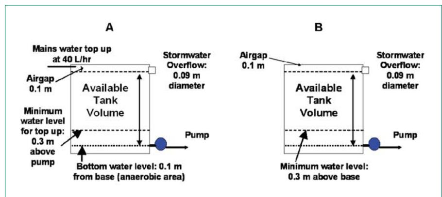
**Figure 2.** Configuration of tanks used in PURRS (A), and MUSIC and Spreadsheet (B).
